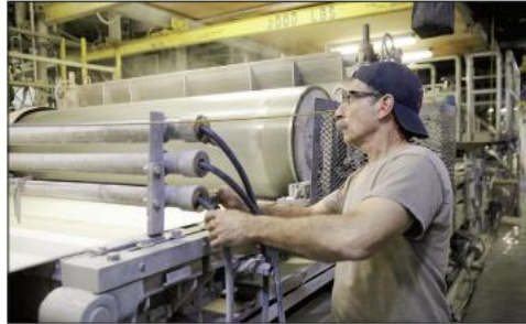
Paul Bianco widens the mold of a paper-making machine at Onyx Specialty Papers in Lee.
